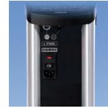
RTC-C reference temperature calibrator with input for reference sensor and DLC sensor.
