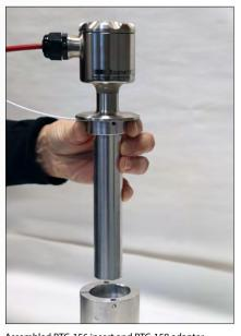
$\label{eq:assembled} Assembled \ RTC\text{-}156\ insert\ and\ RTC\text{-}158\ adapter.$
